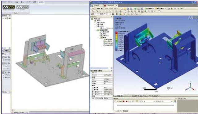
Static structural analysis of a production fixture using SpaceClaim and ANSYS.
